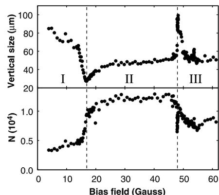
**Fig. 4.** Vertical extension ( $1/e$  half-width of a Gaussian fit) and atom number  $N$  of the expanding cloud as a function of the variable bias field applied in the first 10 ms after release. The measurements are taken after a total expansion time of 50 ms. The three different regions refer to (I) negative scattering length; (II) positive scattering length; and (III) a regime dominated by narrow Feshbach resonances, a prominent one at 48 G and a weaker one at 53 G.
