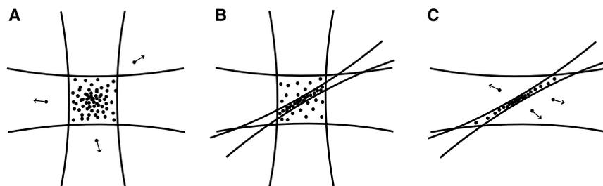
**Fig. 1.** Illustration of the three stages of evaporative cooling toward BEC of Cs. (A) Ten seconds of plain evaporation in two crossed CO<sub>2</sub> laser beams at a magnetic bias field of 75 G (scattering length tuned to 1200  $a_0$ ). (B) Five seconds of collisional loading of a tightly focused 1064-nm laser beam at 23 G (300  $a_0$ ). (C) Forced evaporative cooling by ramping down the power of the 1064-nm beam over 17 s, with the magnetic bias field kept at 23 G.
