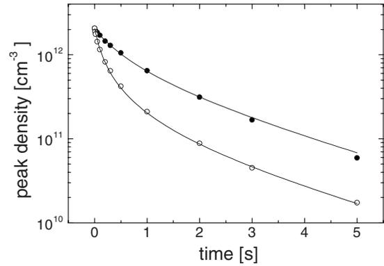
FIG. 17. Time evolution of the peak atomic density in a cloud of  $^{133}\text{Cs}$  atoms in the  $|f=4, m=-4\rangle$  state at  $T=5.3 \mu\text{K}$ . The solid circles show the off-resonant evolution at  $B=140 \text{ G}$ , whereas the open circles show the on-resonant evolution at  $B=205 \text{ G}$  (open circles), where a Feshbach resonance is located. The fit is based on Eq. (55) with  $L_3=0$  and the peak density corresponds to  $2\sqrt{2}\bar{n}$ . From Chin, Vuletić, *et al.*, 2004.
