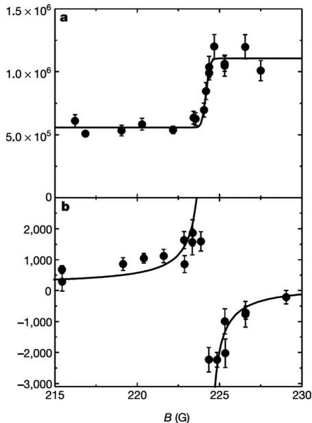
FIG. 32. Molecule formation in a  $^{40}\text{K}$  gas near the 224 G Feshbach resonance. (a) The number of atoms measured after a ramp across the resonance as a function of the final magnetic field shows the disappearance of atoms having formed molecules. (b) For comparison shows the magnetic field dependence of the  $s$ -wave scattering length in units of the Bohr radius, as measured by radio-frequency spectroscopy. From Regal *et al.*, 2003a.
